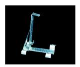
It is produced from flat steel  $40 \times 4$  mm and  $40 \times 2$  mm. It is used for an instalation of Snowguard Ladder on the roofing Onduline. It is hot galvanized.
