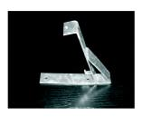
Snowguard Bracket - lower - must be fastened to Base Plate. It is used for Snowguard Ladder. It is hot galvanized.
