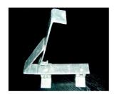
It is produced from flat steel 40 x 4mm. It is used for an instalation of Snowguard Ladder on the roofing with falded metal. It is hot galvanized.
