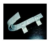
It is produced from flat steel 40 x 4mm. It is used for fixing the Balk on the roofing with falded metal It is hot galvanized.
