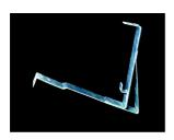
It is produced from flat steel 40 x 4 mm and 40 x 2 mm. It is used for an instalation of Snowguard Ladder on all types of burnt and concrete roofing. It is hot galvanized.
