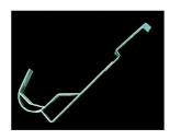
It is produced from flat steel 40 x 4mm and 40 x 2 mm. It is used for fixing the Balk on the metal moulded roofings: CZECOVER, ICOPAL, ONDUSTEEL (š. šablony 408 mm). It is hot galvanized.
